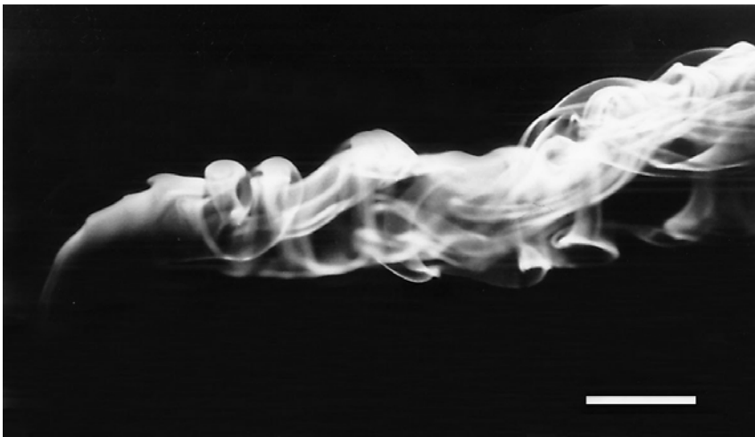
Fig. 10.7. Side view of the turbulent flow of a dye plume in sea water at 1 cm/s over gravel. Scale bar 2 cm. Figure from Weissburg & Zimmer-Faust (1993).
